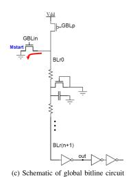
Fig. 3. Circuit schematic for access time simulation.
