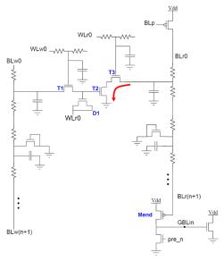
(b) Schematic of cell and local bitline circuit
