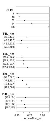
Fig. 5. Association between local bitline access time (ns) and device parameters (number of local bitlines, device lengths (nm)) from Monte Carlo simulations. Parameters are grouped into four intervals. Average access time across Monte Carlo instances within each interval are plotted.
