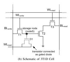
Fig. 1. Comparison of 6T and 3T1D memory cells.
