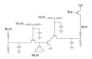
Fig. 2. Circuit schematic for retention time simulation.
